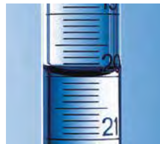
SILBERBRAND Short marks at major graduations. Reading at lowest point of meniscus.
